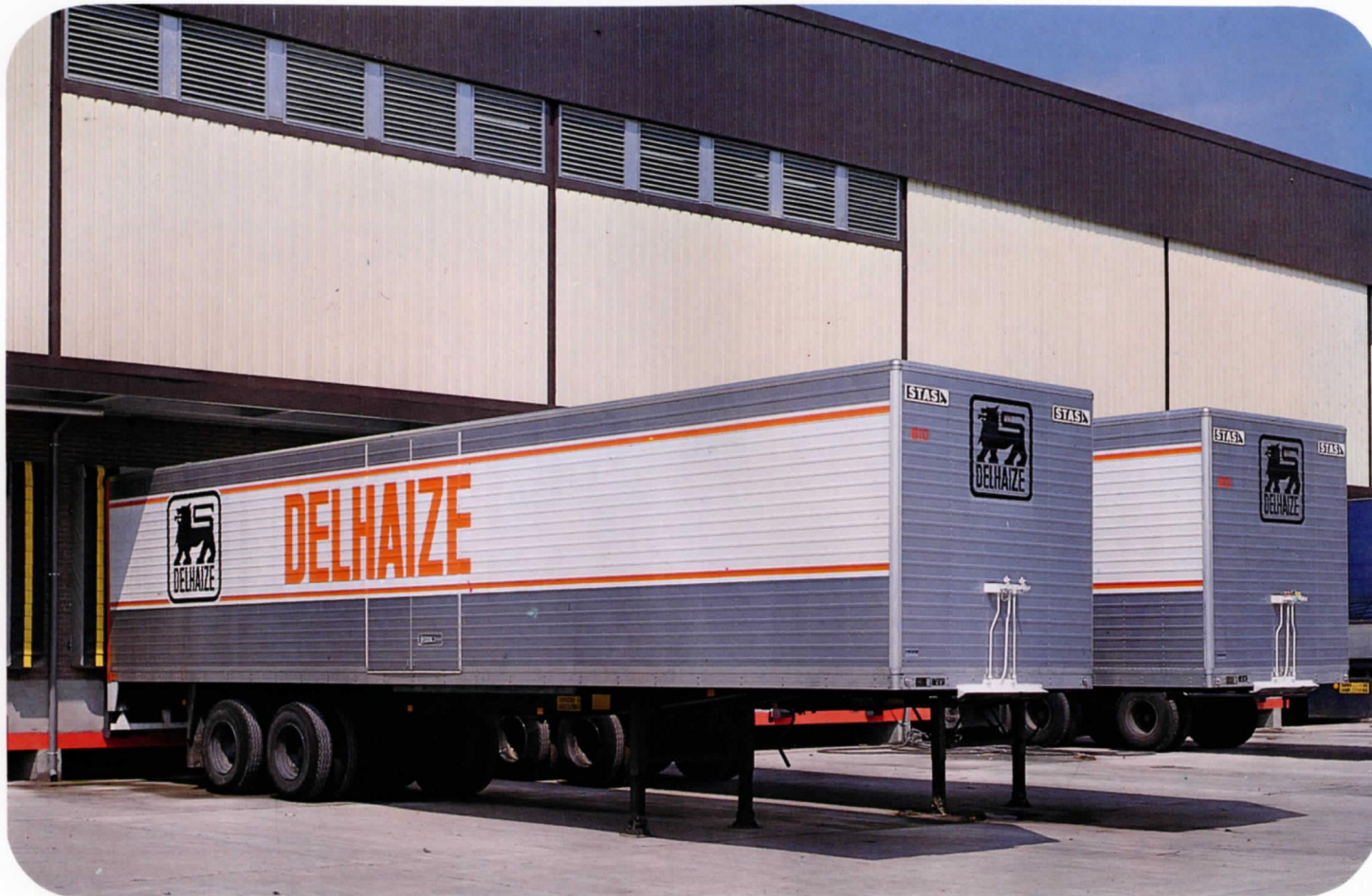
Riveted aluminium semi trailers ALUVAN Semi-remorques ALUVAN en aluminium rivé ALUVAN opleggers in geklonken aluminium
